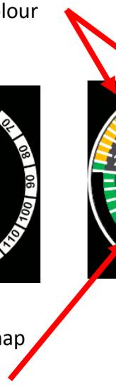
We have already studied how to position the needle and the use of a stripe with a Mask Image, for this case the Total Air Temperature. Now we have a look at the true air speed ring that follows a rotate function.
